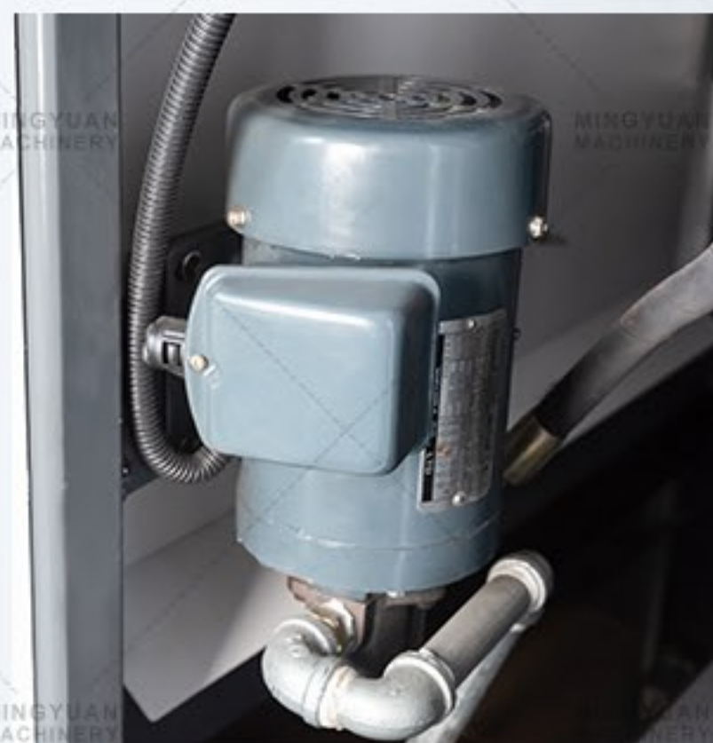
OIL PUMP MOTOR
